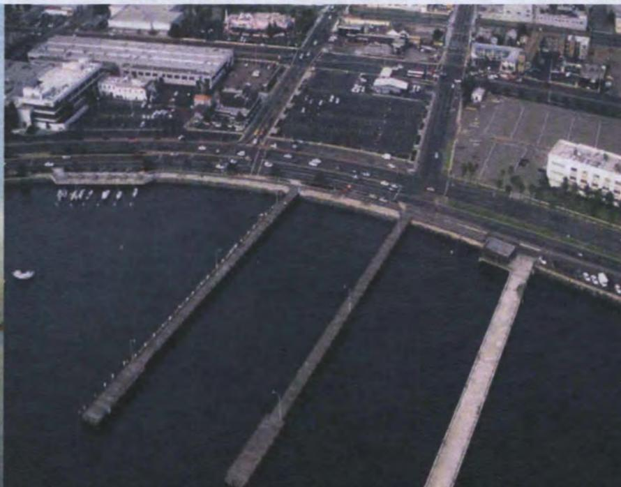
Photo 12. Grape St. Piers (looking east). Pier Nos. 1 and 2 are timber structures in poor condition - formerly used to support the San Diego tuna fleet. Pier No. 3 on the right will was formerly known as "Chevron Pier".
