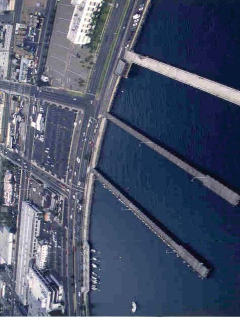
Photo 12. Grape St. Piers (looking east). Pier Nos. 1 and 2 are timber structures in poor condition - formerly used to support the San Diego tuna fleet. Pier No. 3 on the right will be formerly known as "Chevron Pier".
