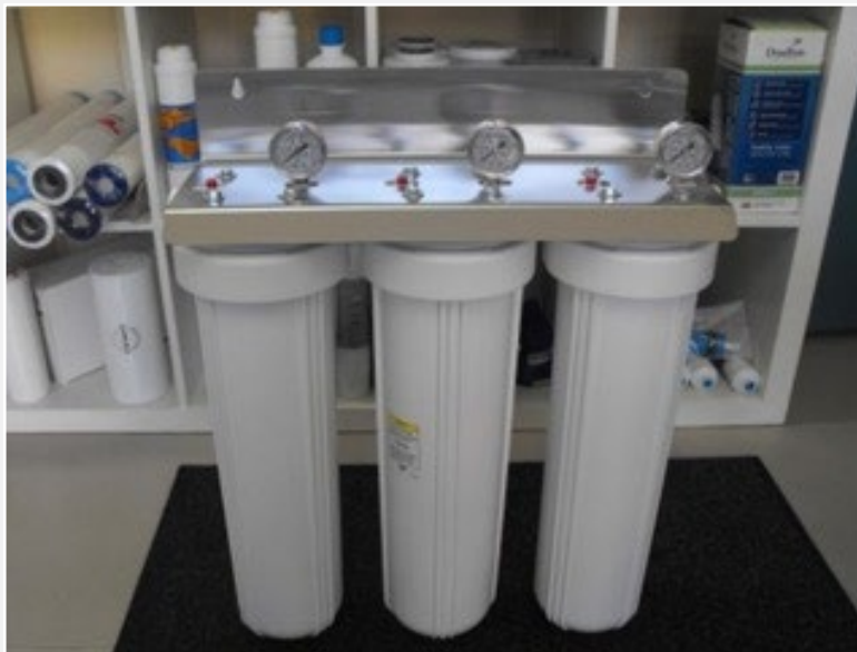
Active filtration device system to be tested in the field using Red Lion patented copper remediation resin technology.
