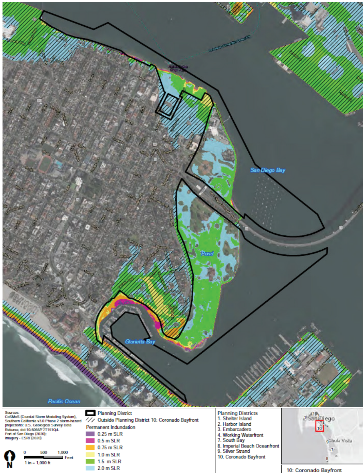
Figure 4.13-8. Permanent Inundation Under Sea Level Rise for Coronado Bayfront (PD10)
