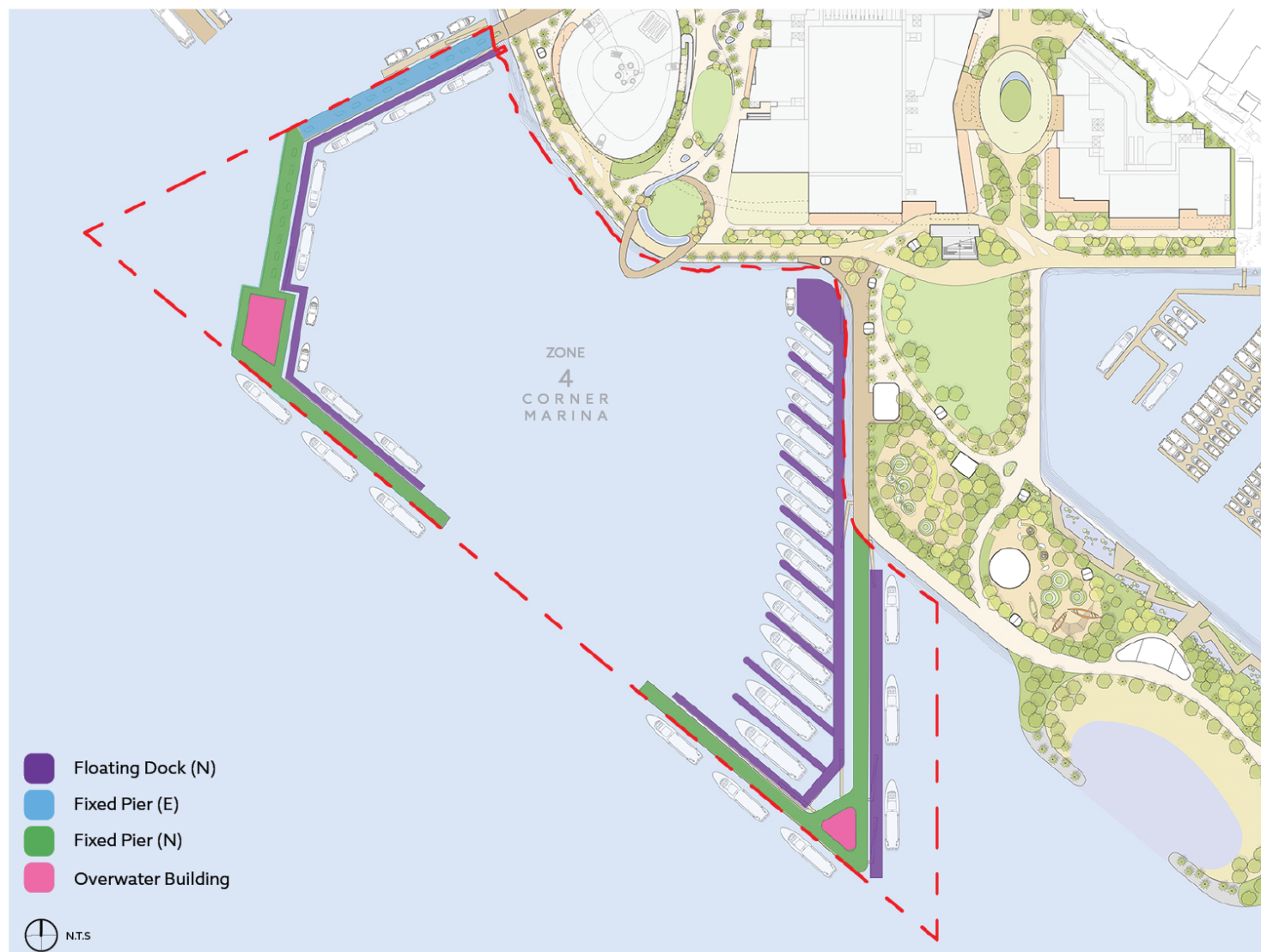
Figure 56. Water-Side Zone 4 Site Plan
