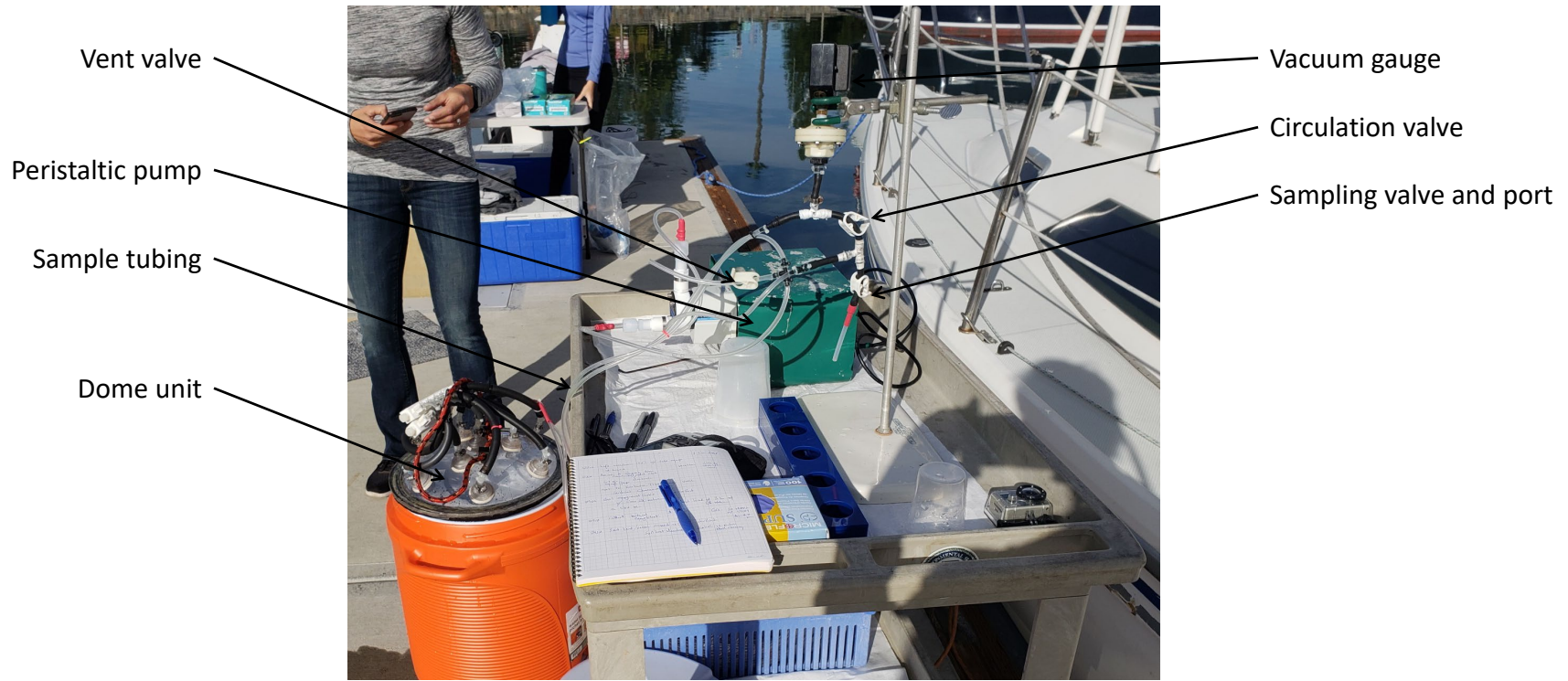
Figure 2-3. Photograph of the dome sampling setup used during the study.
