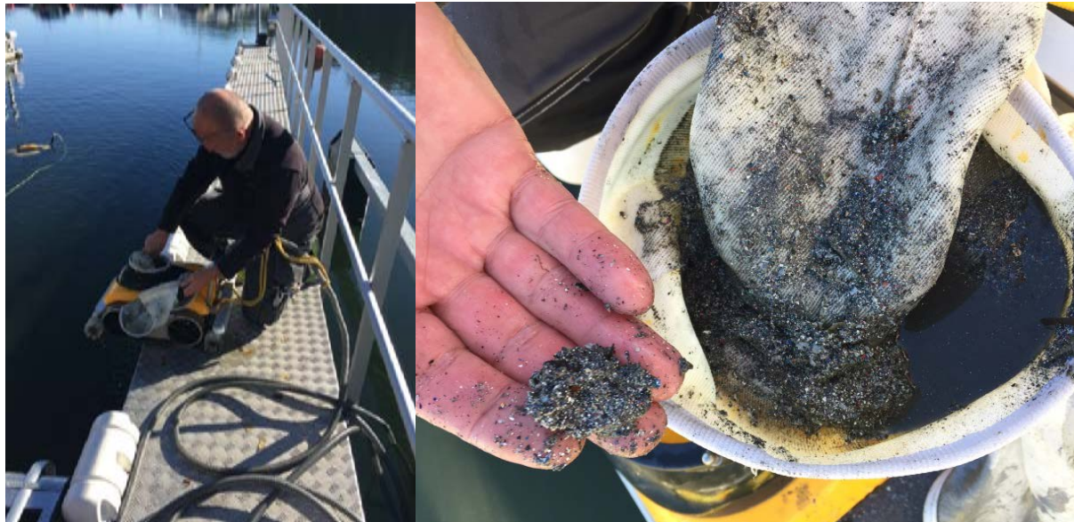
Figure 3-2. Boatwash Vacuum System for the Collection of Particulate Debris and Collected Debris.
