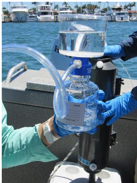
Photo D. Water samples are filtered in the field immediately after collection for analysis of dissolved metals.
