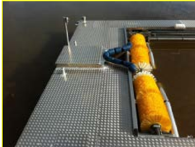
Figure 3-3. Boatwash Cleaning Brush and Arm Configuration.
