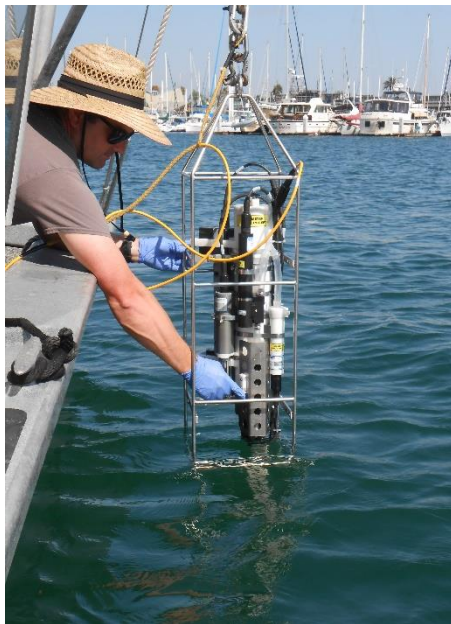
Photo A. Following sample collection, a water column profile of temperature, salinity, conductivity, and transmissivity is conducted using a CTD profiler.
