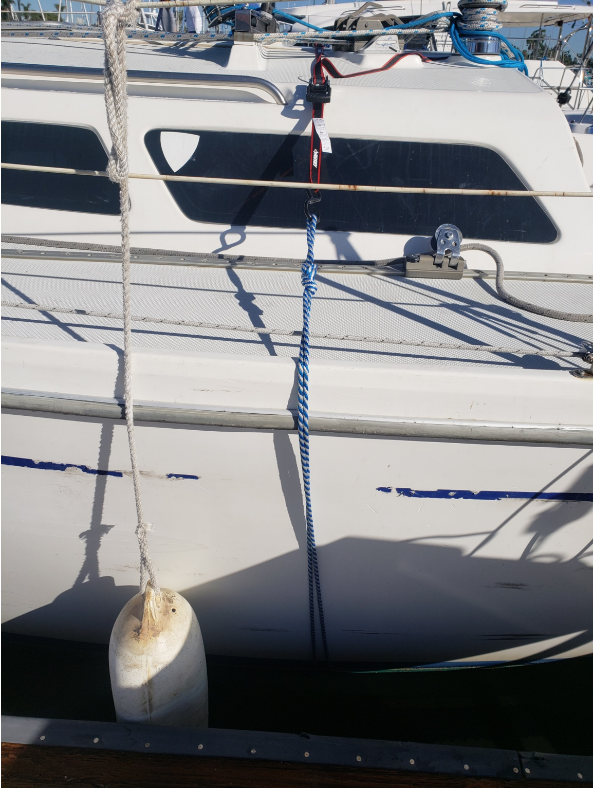
Figure 2-7. Ratchet strap and line used to help secure the dome in place during sampling operations.
