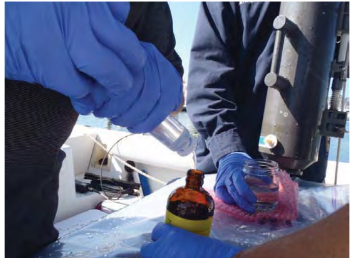
Photo D. Filtration of water samples is conducted in the field immediately after collection for analysis of dissolved organic carbon.
