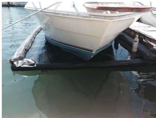
An example of a boat slip liner—a common type of copper-reducing BMP strategy
