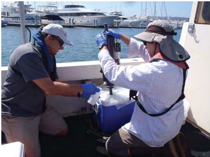
Photo C. Water sample collection for trace level copper analysis using a Niskin bottle following clean sampling techniques.
