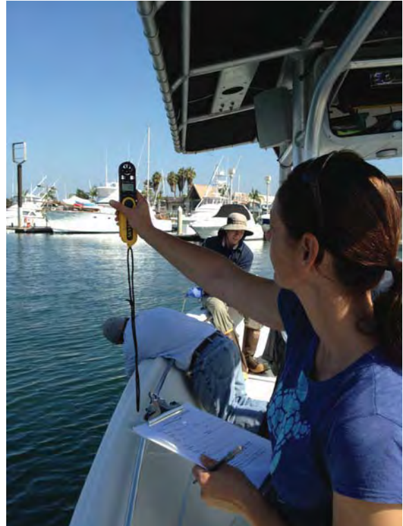
Photo B. Recording of weather conditions, activities such as boat cleaning, and any other observations that may have an impact on water quality is an important component of the field monitoring program.
