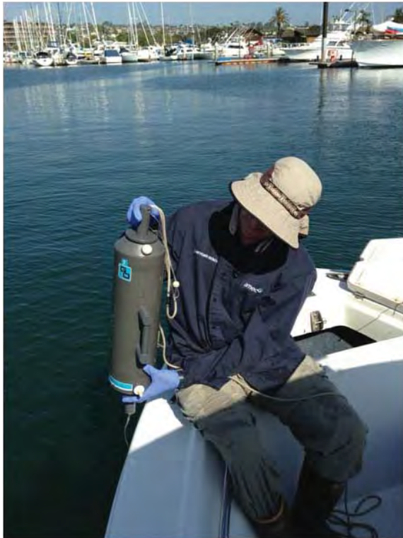
Photo A. Water sample collections were conducted using a Niskin bottle following clean sampling techniques.
