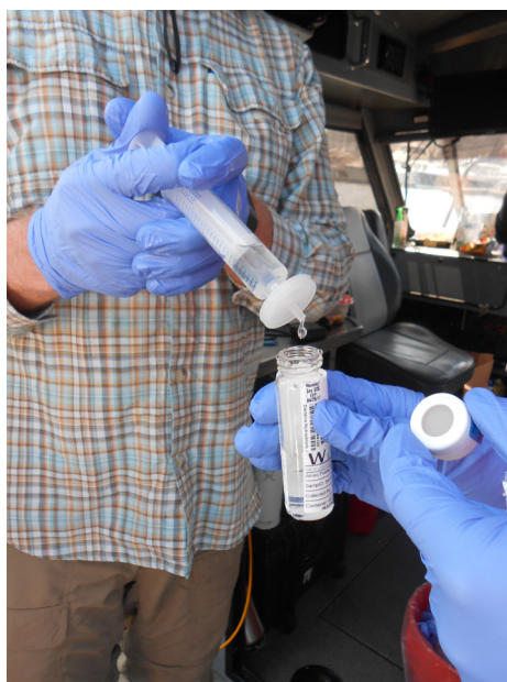
Photo D. Filtration of water samples is conducted in the field immediately after collection for analysis of dissolved organic carbon.
