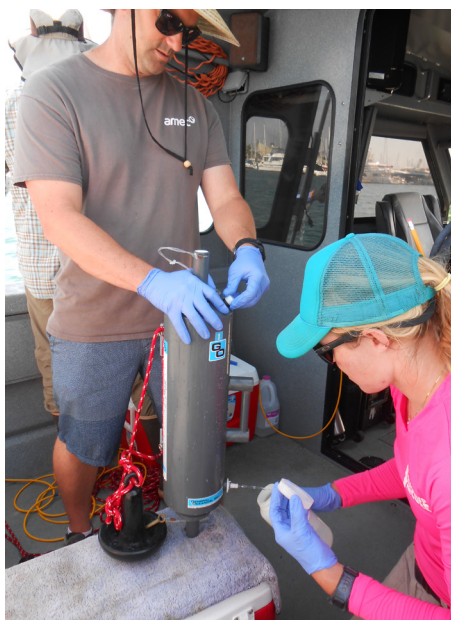
Photo C. Water sample collection for trace level copper analysis uses a Niskin bottle following clean sampling techniques.
