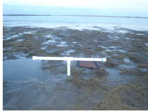
A ceramic tile attached to a PVC tee was used as an oyster spat recruitment collector.
