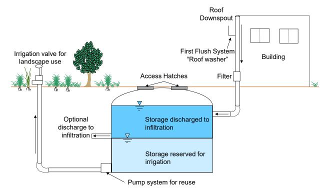
FIGURE 5-6. Schematic of a Typical Cistern
