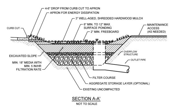
Typical plan and section view of a Bioretention BMP
