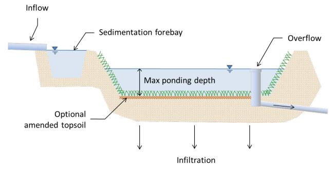
FIGURE 5-7. Schematic of a Typical Infiltration Basin
