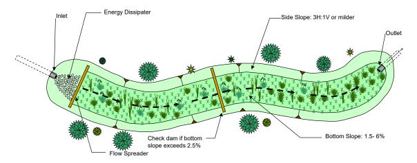
FIGURE 5-10. Schematic of a Vegetated Swale
