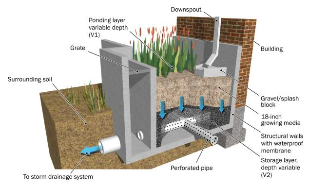
Biofiltration with impermeable liner BMP Example Illustration
