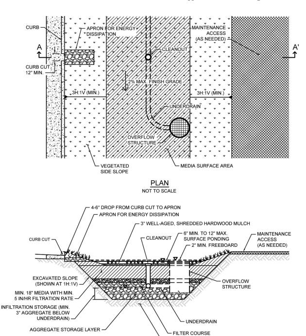
Typical plan and Section view of a Biofiltration with Partial Retention BMP
