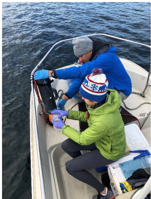
Photo C. Surface water samples were collected using a Niskin bottle and following clean sampling techniques.
