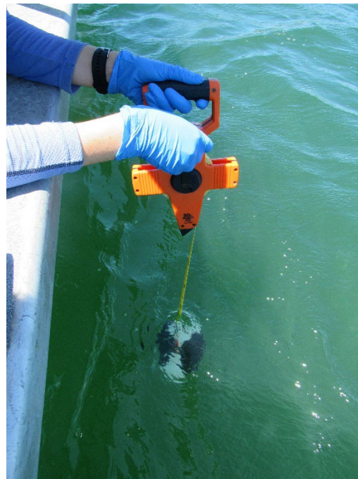
Photo B. Upon arrival at each monitoring station, water clarity was estimated using a Secchi disk (pictured above). In addition, temperature and salinity measurements were taken using a YSI ProDSS water quality meter.
