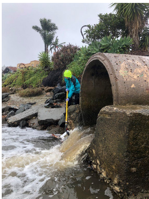
Photo C. Stormwater grab samples were collected from two outfalls (OF-1 depicted in Photo A and OF-2 depicted in Photo C above).
