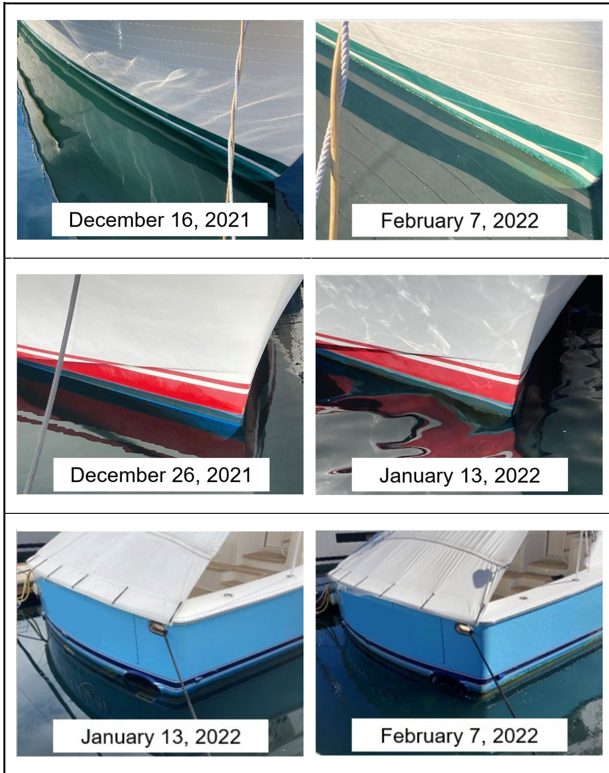
Figure 3-6. Photos of Fouling on Vessel Hulls During the Hull Cleaning Pause
