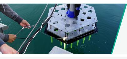
ecoSPEARS deployed clean water technology at two locations in San Diego Bay for a six-month period to address PCB contaminant sediment.
