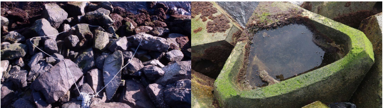
Figure 6. Example of monitoring in the upper tidal area. Left: control rocks marked by a rope; Right: single CL unit.
