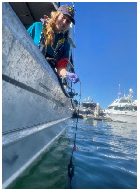
Photo A. Water quality readings of temperature, conductivity, salinity, pH, and dissolved oxygen were taken before, during, and after sampling using a YSI water quality meter.
