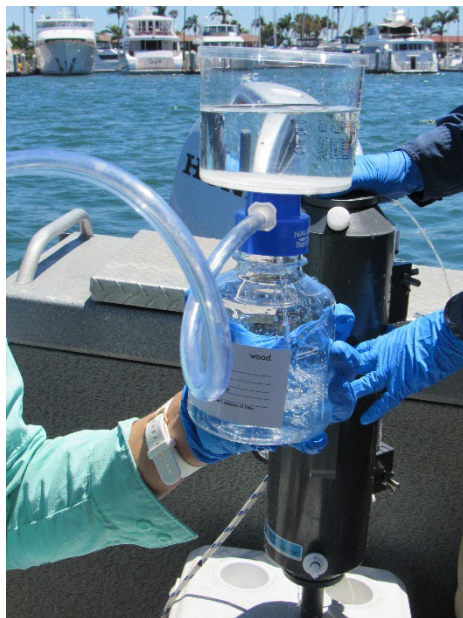
Photo D. Water samples were filtered in the field immediately after collection for analysis of dissolved metals.
