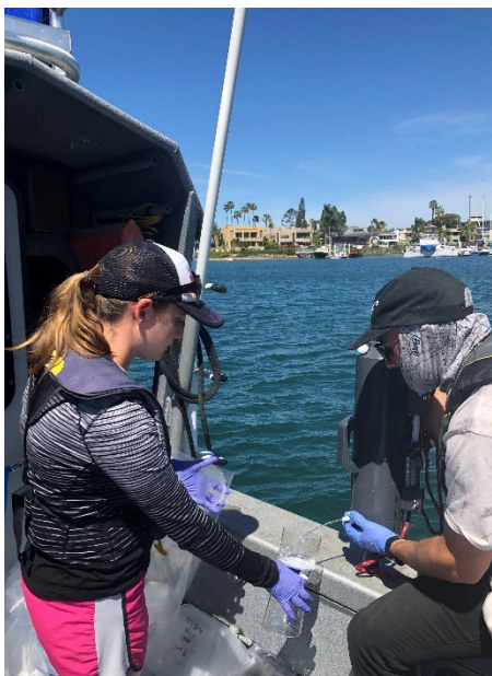
Photo C. Water samples were collected using a Niskin bottle and following SWAMP “clean hands” sampling techniques.
