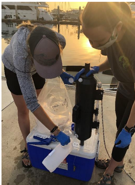
Photo C. Water samples are collected using a Niskin bottle and following clean sampling techniques.
