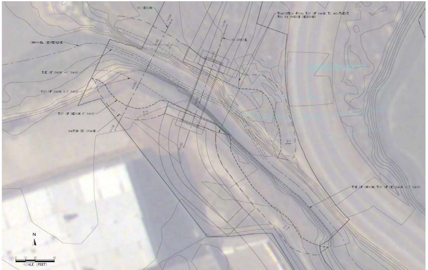
Figure 7-3: Channel and Bench Grading Concept Plan View
