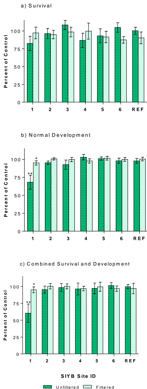
Figure 1. Results of the 48-hour larval bivalve survival and development test for each undiluted sample, a) survival, b) normal development, c) combined survival and normal development; presented as the mean result ( \pm one standard deviation) normalized to the control. Note: all three endpoints are displayed separately here for additional information, but only the combined endpoint is used for NOEC/LOEC determination and TST pass/fail calculations. A single asterisk (*) indicates a significant decrease compared to control using the traditional EPA flow chart statistical methods, a double asterisk (**) indicates a significant decrease with both EPA flow chart methods and the TST.
