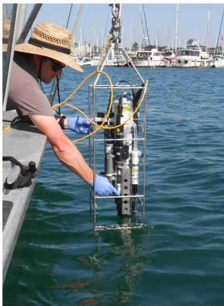
Photo A. Following sample collection, a water column profile of temperature, salinity, conductivity, and transmissivity using a CTD profiler.
