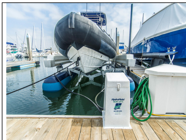
BMP copper-reducing strategies such as the Hydra Hoist® (left) and dry space storage (right)
