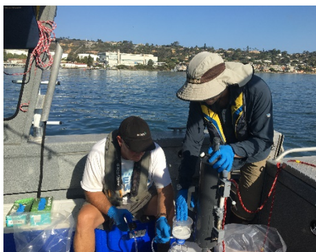
Photo C. Water sample collection for trace level copper analysis uses a Niskin bottle following clean sampling techniques.
