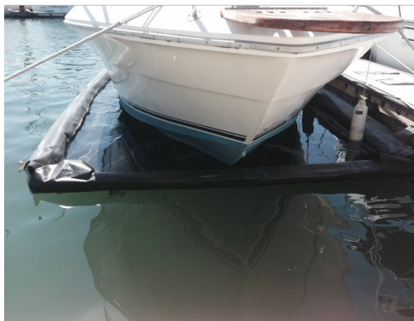
An example of a boat slip liner – a common type of copper-reducing BMP strategy
