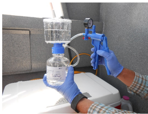
Photo D. Filtration of water samples is conducted in the field immediately after collection for analysis of dissolved metals.
