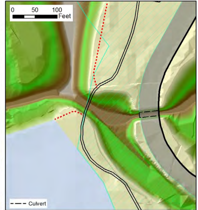
Alternative 3: Expand and Deepen Channel, Add Additional Culvert, and Construct Bridge for Multipurpose Trail/Bikeway
