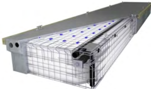
Concrete float concept design mockup
