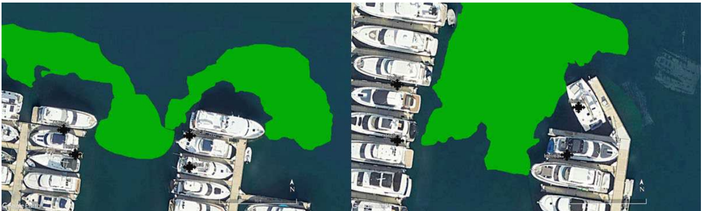
Figure 3. Zoomed in map of eelgrass and helical anchor placements. In this image, black multidirectional arrows represent anchors. A different symbol was used to stand out more in the higher resolution map.
