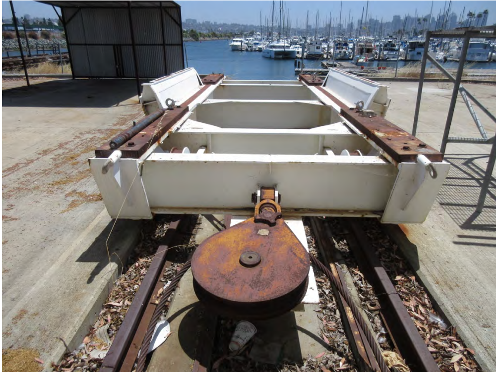
Photo 11: Steel rail car used to move the Deep Quest submarine, looking east.
